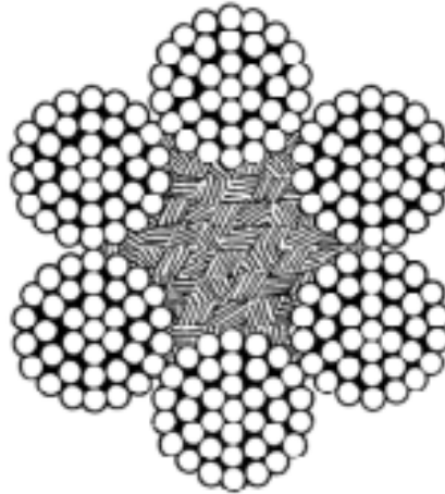
Fig. 5 – Cable 6 x 37 + T (alma textil)
